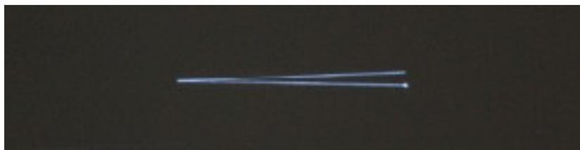
If the angle is greater, you adjusted the azimuth the wrong way. If the angle is reversed (the initial star point is now above the lines), then you adjusted the azimuth too much. Continue to make adjustments to the azimuth on the mount until you image looks like the image below.
